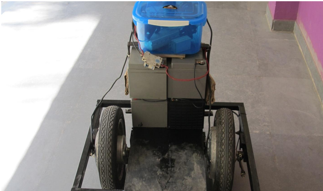
Fig4: This is the battery pack of the fail-safe segway personal transporter
