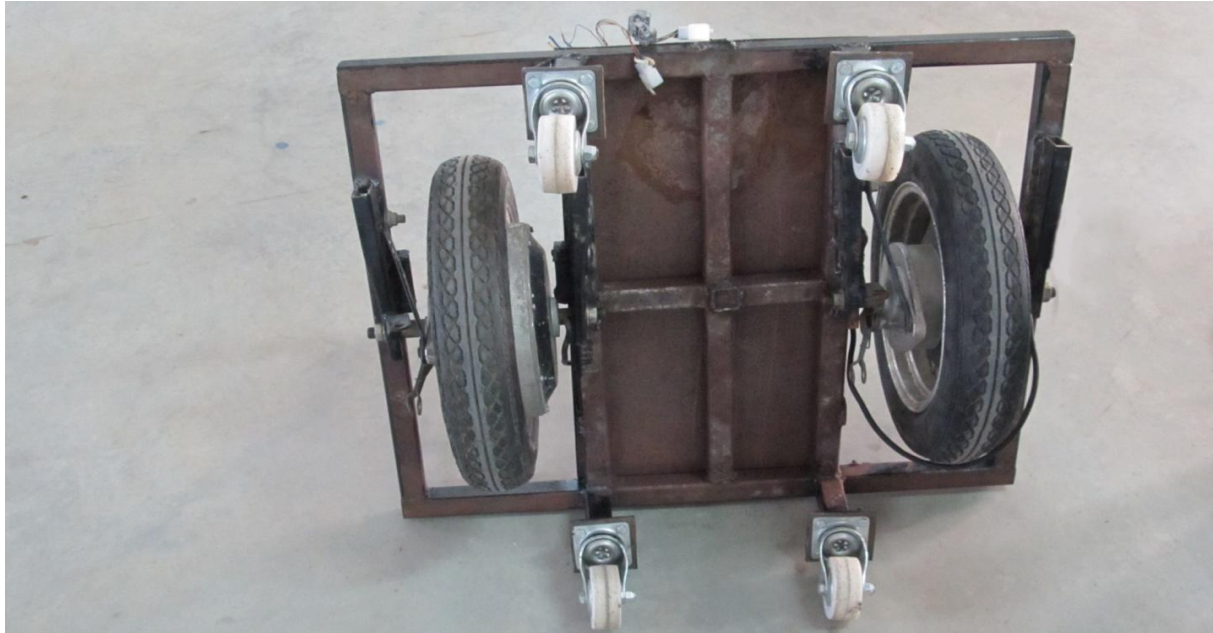
Fig2: Frame and supporting wheels of the fail-safe segway personal transporter
