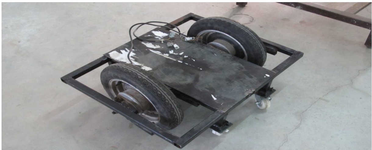
Fig1: Frame of the fail-safe segway personal transporter
