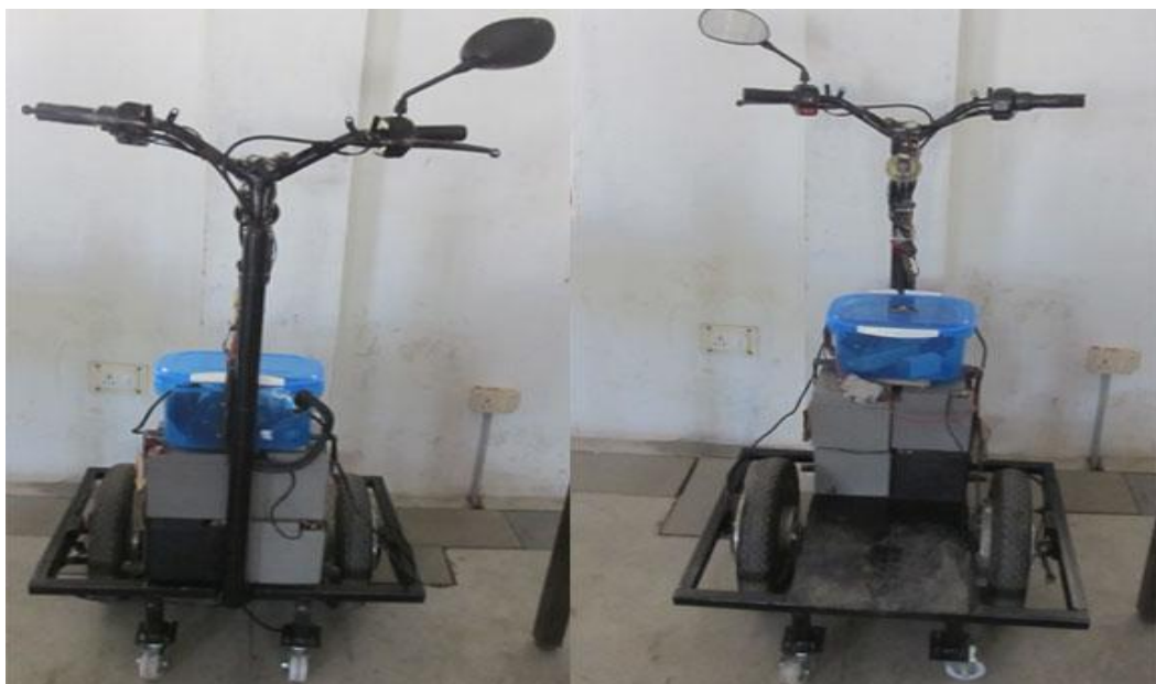
Fig5: The fully fabricated fail-safe segway personal transporter
