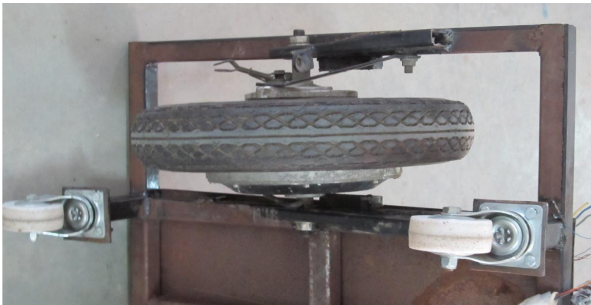
Fig3: The In-hub motor of the electric scooter
